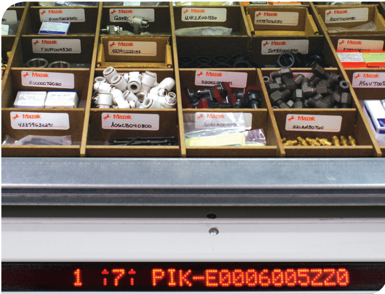
Pick lights light on Shuttle VLMs direct the operator to the exact location, and display the part number and quantity to pick.
