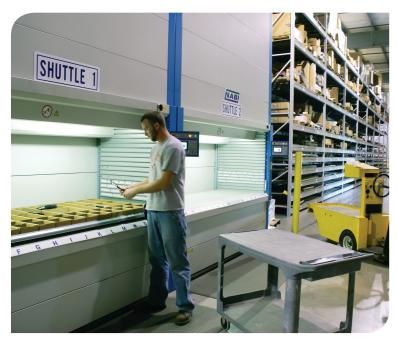
The Shuttle VLM, delivers parts to the operator at an ergonomically correct height with just a push of a button creating a safe work environment.
